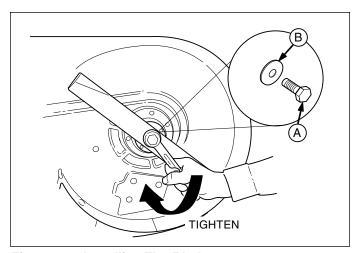
Figure 9. Installing The Blade
